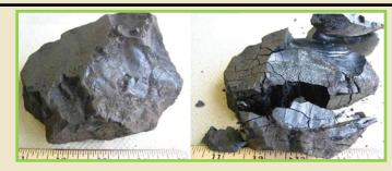
"This 5-day-old undisturbed coal fractured simply as a result of exposure to oxygen and the rapid decrease in moisture content. As a result, combustible dust can easily be dispersed into the air and, when exposed to oxygen and a source of ignition, may become a significant danger. (*Power Magazine*, 2011)
